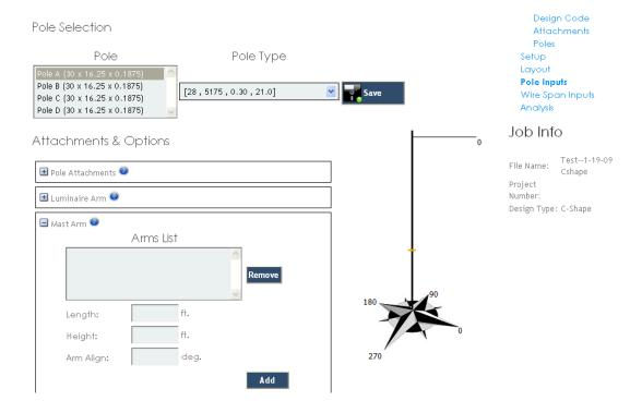
The length of the mast arm, height and angle of orientation are the only inputs needed for the arm. The dimensions of the mast arm are estimated from the length that is specified. After adding the arm, attachments can be placed along its length. To place attachments, select the arm from the arms list and then proceed to pick the attachment type and distance from the face of the pole. As the user inputs the arms and attachments, the image will update showing the placement.
