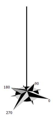
When wires are attached to the pole, one of the wires will have a hard coded angle applied to it. All attachments should be placed in relation to this wire and the angle that it possesses.
