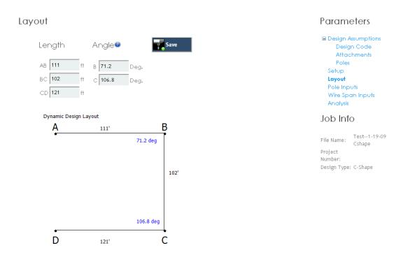
Angles are labeled based on the pole that the wires are attached. For example, Angle A is the angle between the wires at Pole A. Angles must add up to 360 for a Box and Drop Box configuration and 180 for a Triangle configuration.
